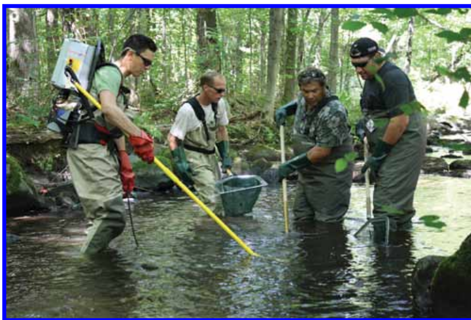
Backpack Electrofisher Stuns Fish for Capture to Assess Fish Populations in the Stream
