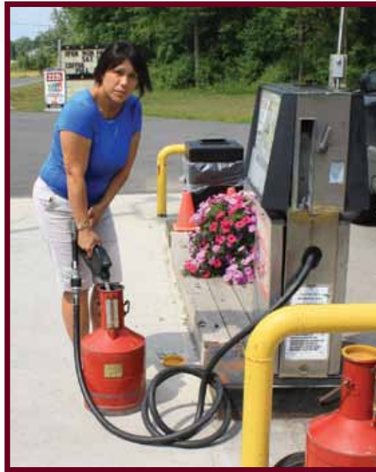
Inspector Carrie Benedict Dispenses Fuel to Verify Proper Accuracy
